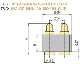
Replace NNN by the number of poles, standard number of contacts 2 to 20 contacts. See table below for ordering number according to height and working range.
