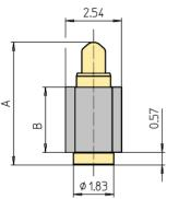
INSULATOR: Black glass filled polyester PCT-GF30-FR DYNAMIC CONTACT RESISTANCE: 20mΩ OPERATING TEMPERATURE RANGE: -55/+125 °C COPLANARITY SMD: 0.1 mm (on 25 mm long) DURABILITY: 20'000 cycles OPERATING CURRENT: Max 5 A
